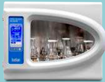
ES-20/80, Orbital Shaker-Incubator
