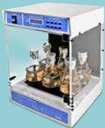
ES-20, Orbital Shaker-Incubator
