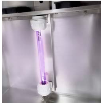
Air UV recirculation system in the chamber
