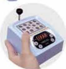
Clear block cover ensures temperature uniformity
