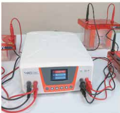
Four pairs of outlet terminals
