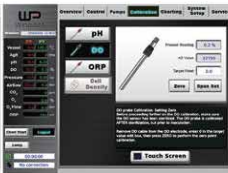
Online system calibration with system feedback
