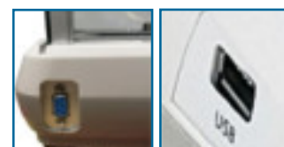
RS232 & USB port for Printer, PC & flash drive connections
