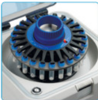
Stainless steel, 24 position tube carrier
