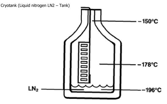
If vials are to be immersed in the liquid phase of liquid nitrogen, they must be correctly sealed. Improper use may cause entrapment of liquid nitrogen inside the vial and lead to pressure build up, resulting in possible explosion or biohazard release. Liquid phase LN penetration can also be a source of
