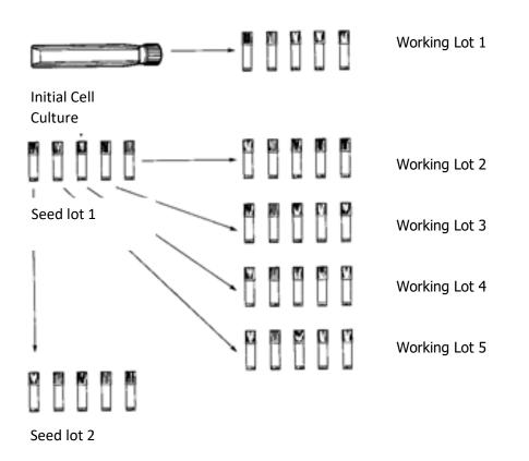
When the first lot of working stock is depleted, a vial is retrieved from the seed lot and used to prepare a second working stock. This continues until all seed vials, except one have been depleted. The last seed vial is then used to prepare a second seed lot. The second seed lot remains only one or two passages from the original material, but may be separated by many years if the lots are adequately sized
