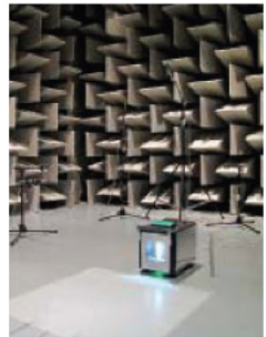
ISO 3744 acoustic test
