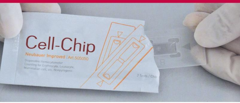
The counting chamber looks like the familiar Neubauer "improved" hemocytometer: The cells are distributed over  $3 \times 3$ large squares, each with 1 mm edge length and with a surface area of 1 mm<sup>2</sup>.
